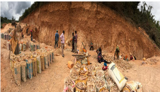
Figure 2: Crushing site showing aggregates packed in the used cement bags
